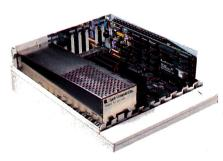
RamKeeper is easy to install and stores programs in an "instant on" electronic bard disk.
